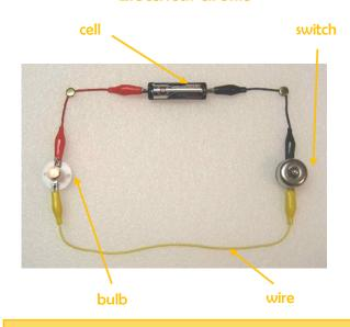
The switch opens and closes the circuit. The bulb lights in this circuit because the switch is on.
