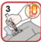
PUSH DOWN HARD until a click is heard or felt and hold in place for 10 seconds
