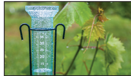
A rain gauge measures precipitation .
