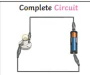
Electricity can flow. Components will work.
